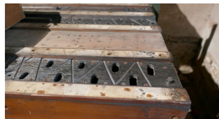
The Great chest at Shirley with sliders and upper boards removed. The zig-zag grooves are to allow air to bleed away from adjacent pipes if the lower and upper boards contract. The grooves were insufficient and holes had to be punched in the toshing underneath the chest to allow excess air to escape.
