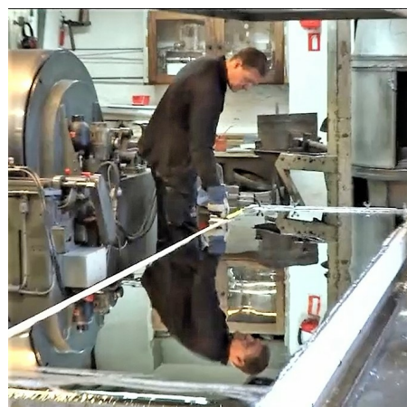
Clips from the video recorded at the Marcussen Organ factory in Aabenraa showing the rarely seen process of pouring and spreading pipe metal into a uniform layer.
