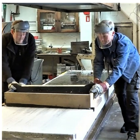
Clips from the video recorded at the Marcussen Organ factory in Aabenraa showing the rarely seen process of pouring and spreading pipe metal into a uniform layer.
