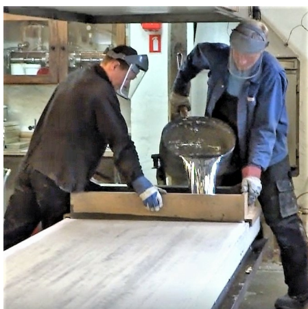
Clips from the video recorded at the Marcussen Organ factory in Aabenraa showing the rarely seen process of pouring and spreading pipe metal into a uniform layer.
