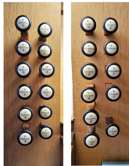
Frobenius stops: note the letter 'B', 'G' and 'P' to identify the Brustpositive, Great and Pedals.
