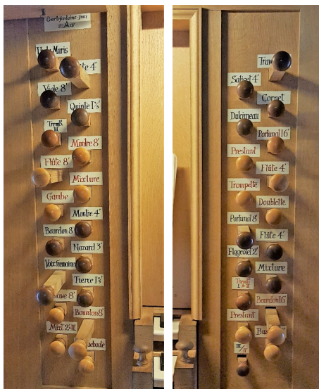
Aubertin stops: note the colours of the stops and labels to identify the manuals and pedals.
