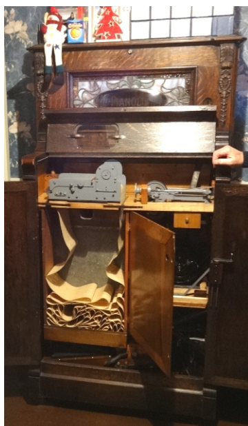
'Pianolin', coin operated piano from New York c.1920 contains a 44 note piano mechanism together with 44 'violin' and flute pipes. Behind the front doors is revealed a paper roll mechanism in the form of a continuous loop.
