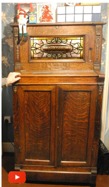
'Pianolin', coin operated piano from New York c.1920 contains a 44 note piano mechanism together with 44 'violin' and flute pipes. Behind the front doors is revealed a paper roll mechanism in the form of a continuous loop.
