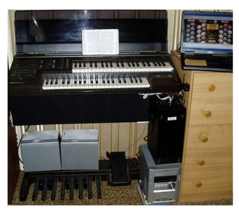
Alan's "shoestring" organ. The silver speakers on the left are two of the four connected to the 100w amplifier (bottom right). The black box on the right is the main unit and subwoofer of the Cambridge 5.1 system.
