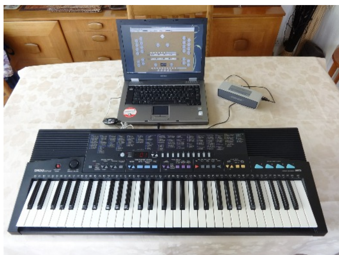
A typical set-up showing a laptop computer, loudspeaker, MIDI to USB connector (on the left of the laptop) and a MIDI keyboard.
