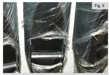
Guy demonstrated the effect of 'nicking' the speaking part of the pipe and the effect on the attack and speech of each pipe. Larger pipes, such as the Pedal Principal, which was on the large voicing chest, have only a token nicking – not simply a sign that the voicer has taken care with each pipe but a subtle change to the attack and speech of each pipe (fig. 5). (Note the cling film used to protect the pipes from finger marks during transit and installation.)
