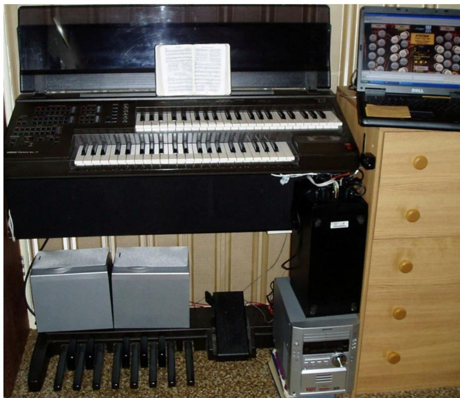
Alan's "shoestring" organ. The silver speakers on the left are two of the four connected to the 100w amplifier (bottom right). The black box on the right is the main unit and subwoofer of the Cambridge 5.1 system.
